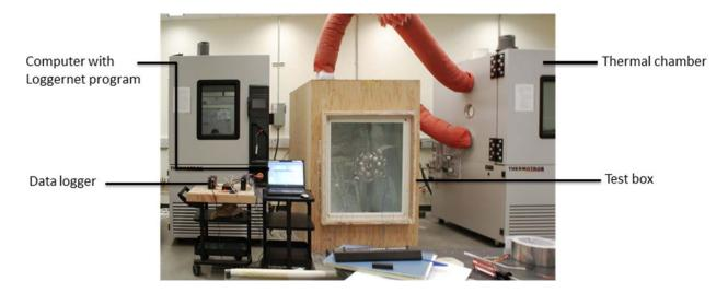
**Figure 1**. Insulated test enclosure located within the Green Building Research Laboratory (GBRL) at Portland State University.
