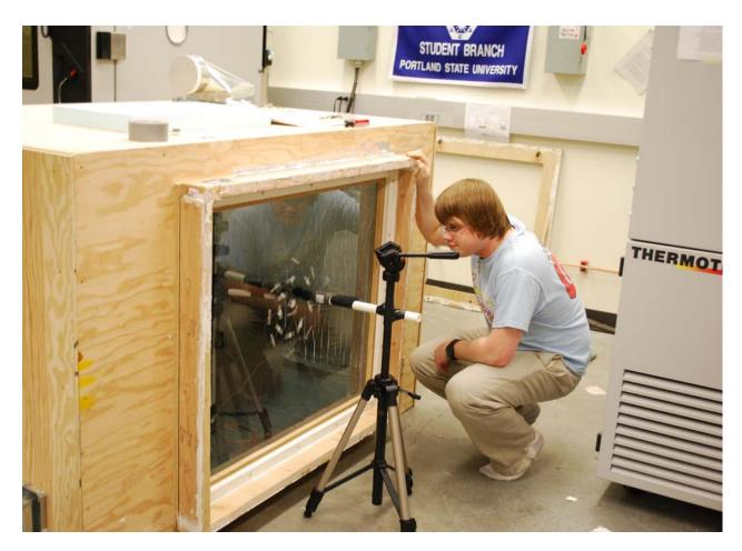
**Figure 3**. Noise abatement testing. Sound source is located at a specified location interior to the test fixture (outside environment) while noise levels are measured by the tripod-mounted microphone located outside the test fixture (inside environment).
