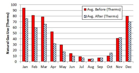
**Figure 13**. Monthly breakdown of measured natural gas consumption (averaged over the 4 pilot homes) before and after the installation of Indow Windows.
