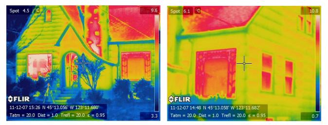
Figure 6. Sample infrared images from the McMinnville pilot home site.
