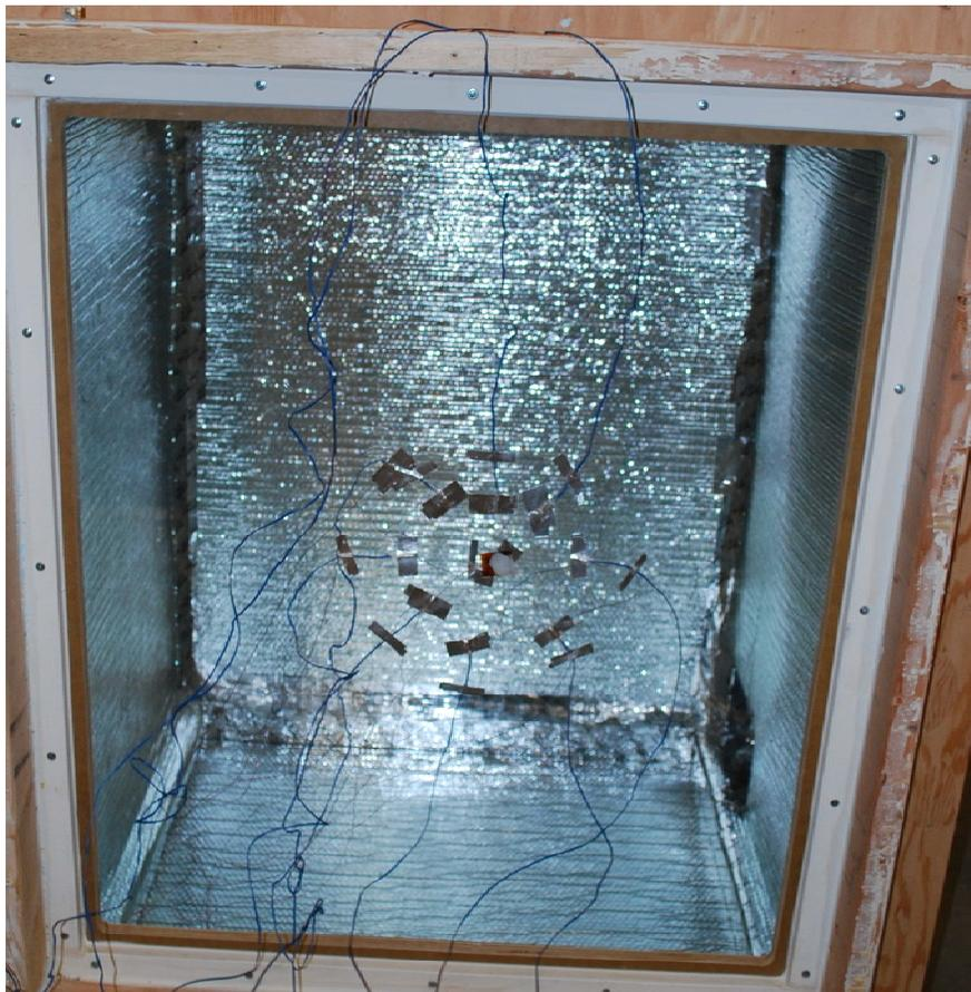
**Figure 2.** Close-up view of the instrumented Indow Window as installed in the thermal test fixture.
