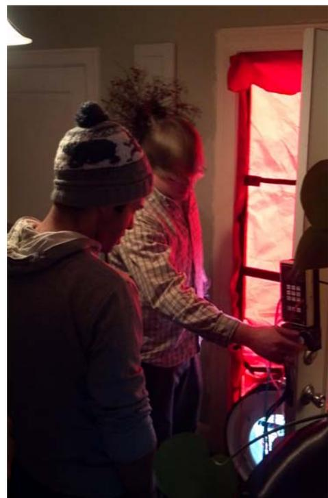
**Figure 5.** Blower door tests being conducted at McMinnville pilot home site.
