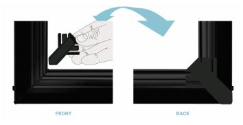
4) Lift PRO frame into primary frame, align
