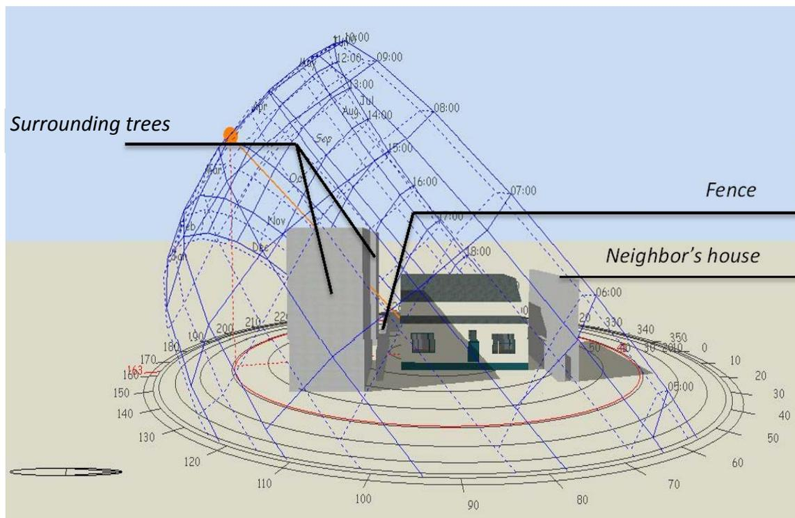
**Figure 8.** Shading of the North Portland house in DesignBuilder (add legend and photo of real shading)
