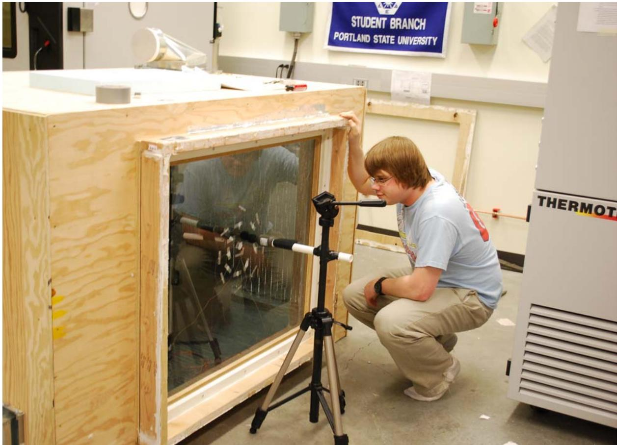
**Figure 3.** Noise abatement testing. Sound source is located at a specified location interior to the test fixture (outside environment) while noise levels are measured by the tripod-mounted microphone located outside the test fixture (inside environment).
