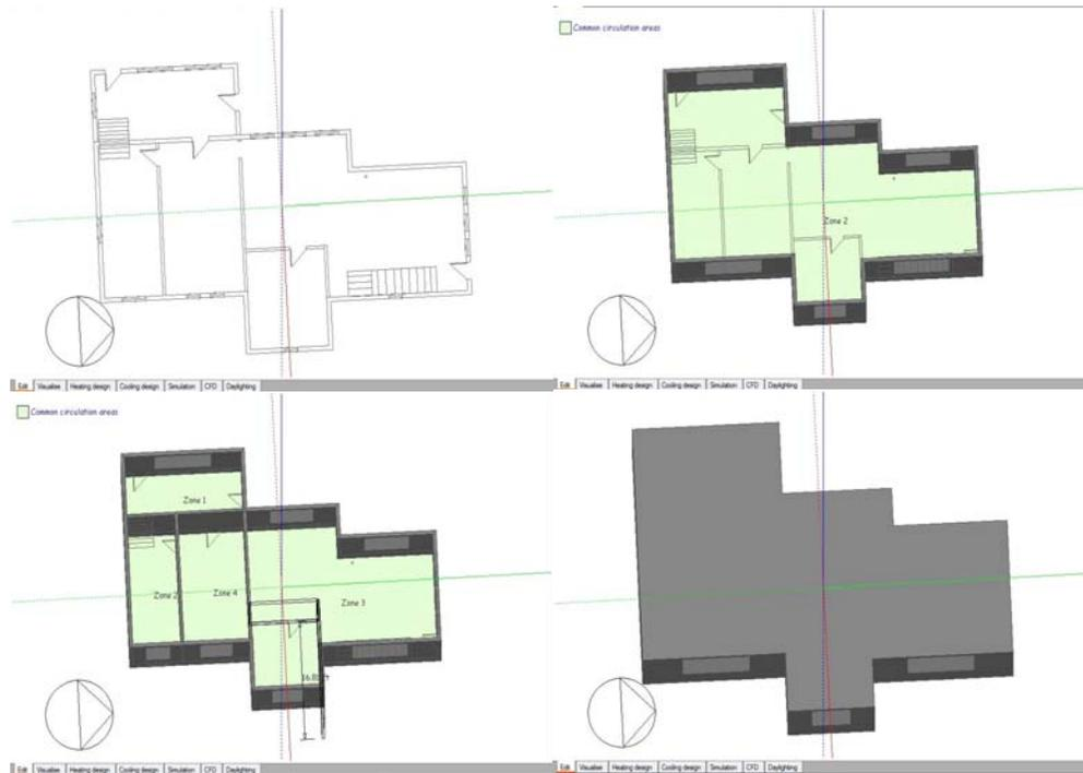
**Figure 7.** Building geometry being extruded from AutoCAD floor plans.
